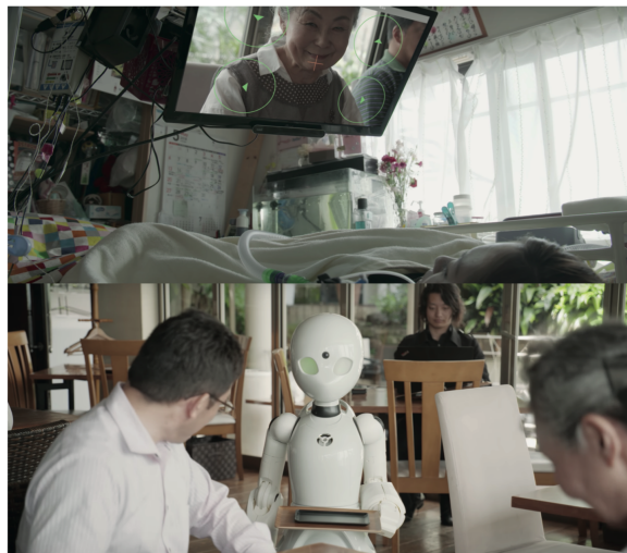
Figure 2: ALS-patient serving customer at OryLab's pop-up cafe. Top: ALS-patient at home sees a live video feed from the cafe. Bottom: The robot waitress at the cafe
